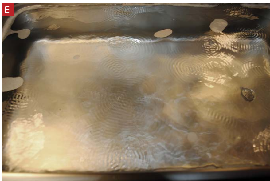
E. Cavitation bubbles are invisible to the eye, but the cleaning tank emits a buzz and the surface ripples from the waves.
