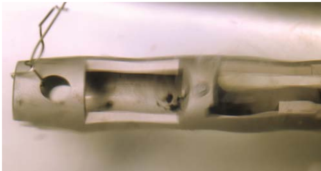
Right: Cleaning progress as seen in this series for the Ruger Mark II barrel suspended horizontally (distortion is from surface waves). From top to bottom: before the unit was turned on; one minute into the cleaning; after 5 minutes. Note the carbon accumulation, illustrating why areas where crud can accumulate need to be blown out or mechanically cleaned.
